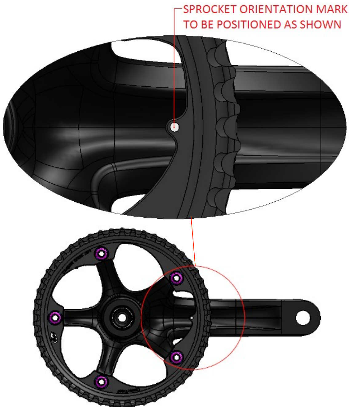
Figure 1: Tab mounting location for correct sprocket orientation.
