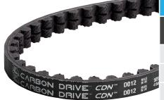
The CDN belt has nine carbon cords embedded within an engineered polymer belt with a patented 11 mm tooth pitch profile optimized for lower tension.
