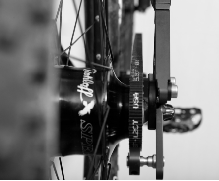
Illustration 3: Correct alignment of the belt
