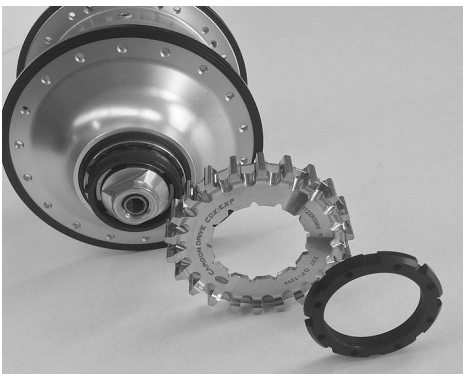
Illustration 1: Rohloff SPEEDHUB 500/14 with Splined Carrier and Lock-Ring
