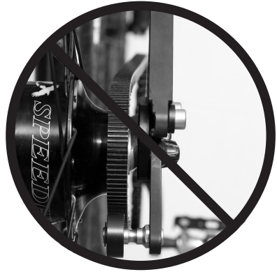
Illustration 4: Incorrect alignment of the belt
