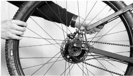
Illustration 3: Correct alignment of the belt
