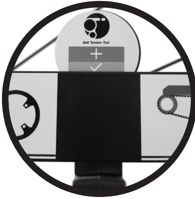
Illustration 3: Optimal belt tension
