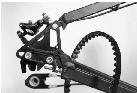
Illustration 1: Opening the frame to mount the belt
