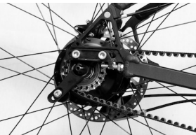
Illustration 3: Side view of the installed Snubber
