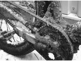
Illustration 1: The Gates Carbon Drive System used in a muddy environment
