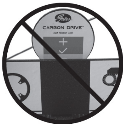
Figure 2: Tension excessive de la courroie
