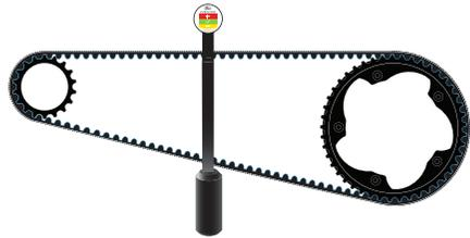
2 Put the ruler on the two sprockets. Check the tension:
