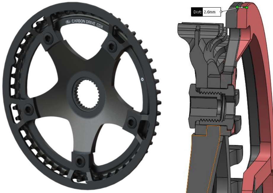
The guard shown in red will be replaced with a narrower guard, adding 2.6mm of outboard clearance.
